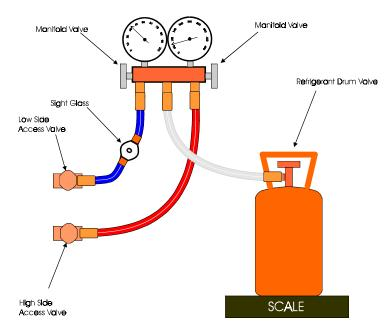
Hose Connection Schematic for Liquid Charging
