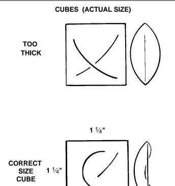
Note: Optimum performance will be achieved when the ice machine is adjusted to produce this size and shape of cube. The typical batch weight at this setting is between 8.25 and 9 pounds.
